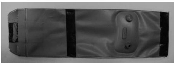
**Fig. 5.48** Pressure bladder for automatic occlusion pressure controller
