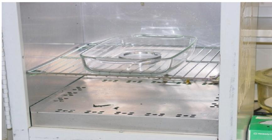
**Fig. 2.44** Water vapor transmission cup in constant temperature oven, 37°C
