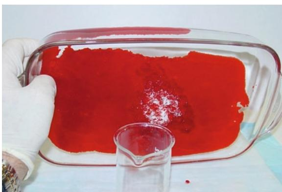
**Fig. 2.37** Demonstration of efficient absorbance of porcine blood after 30 s by holding the tray vertically showing a solid nonfluid mass that adheres to the glass tray
