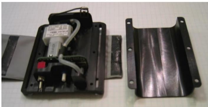
**Fig. 5.49** Automatic occlusion pressure controller, with pressure bladder attached, *inside view*
