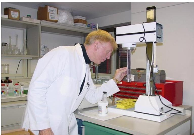
Fig. 4.2 Silverson Homogenizer machine used for shearing liquid in water to form emulsions
