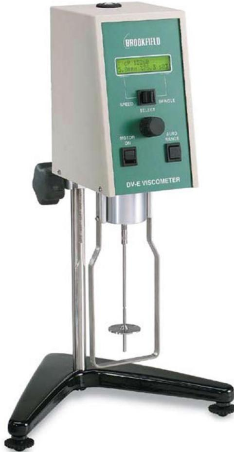
**Fig. 4.4** The Brookfield Viscometer (Model DV-E) is a revolving spindle in a liquid type instrument
