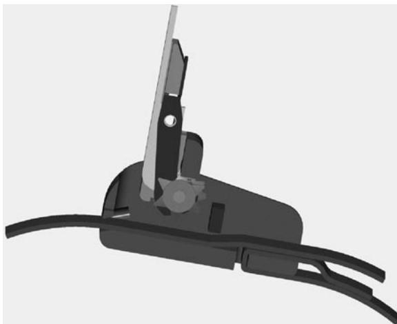
**Fig. 5.33** Cinch buckle open to adjust strap, *cut-away view*
