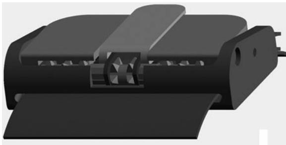
**Fig. 5.34** One-hand cinch buckle closed to secure strap
