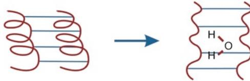
Fig. 2.20 Expansion between polymer chains with interaction with water
