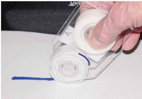
**Fig. 2.56** Demonstration of barrier dressing removal (*blue*) by reverse-side pressure-sensitive tape and roller; note that the dressing remains on the tape and protects the substrate from further exposure to the dressing after removal; the tape can be safely disposed after use
